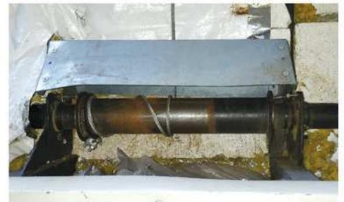
Cables tend to walk all over the lift drum and cause problems
